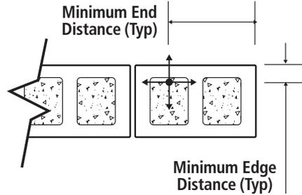
**Allowable Load Capacities for UltraCon+ Anchors Installed in Clay Brick Masonry<sup>1,2,3,4</sup>**
