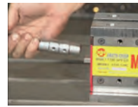
Switch-connect vises to turn them ON/OFF in unison.
