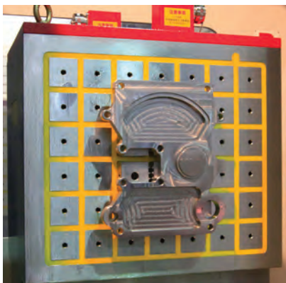
Complex part shapes - 5 sides machining
