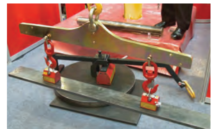
Spreader bars are used for long or very heavy loads
