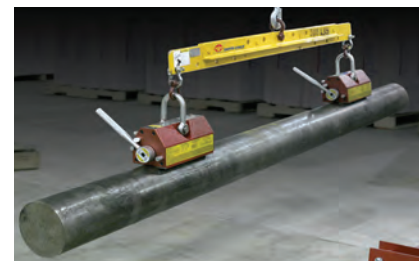
Use spreader bar for improved versatility
