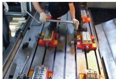
Lock them in position using bolts provided
