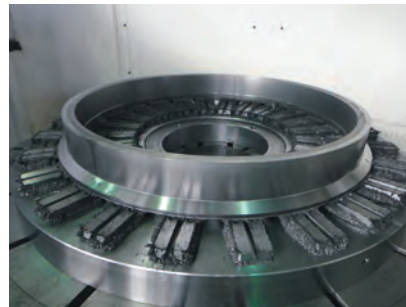
Even workholding - no part distortion
