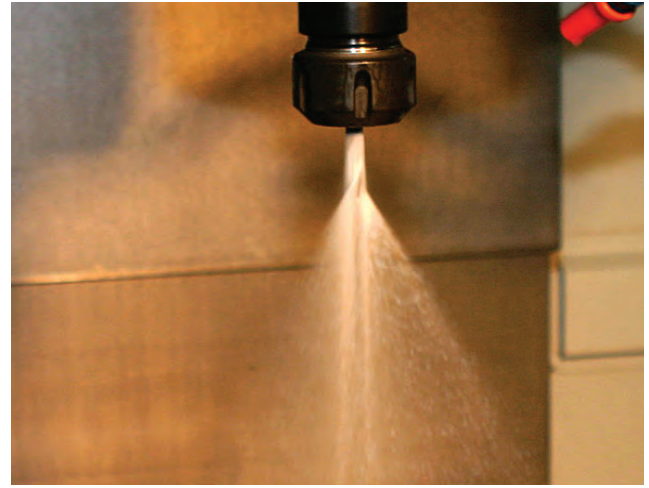
Removing the o-ring creates a CoolBLAST coolant effect.
