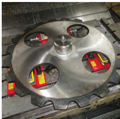
Large tooth sprocket being machined
