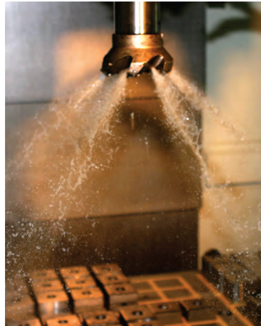
CoolBLAST arbor screw provides coolant path.
