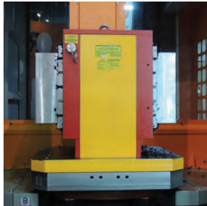
2-sided EETM on palletized system
