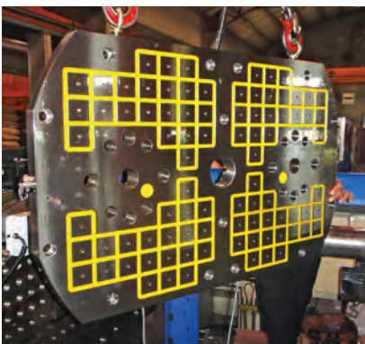
Load and install PIM magnet with bolts
