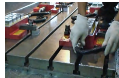
Connect the control cables to chucks and control
