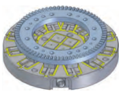
circular chuck setup for gear cutting
