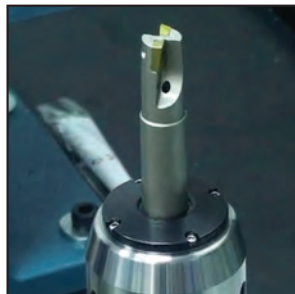
Coolant-thru tool installed
