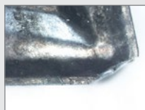
Breakage (Mechanical Wear)
