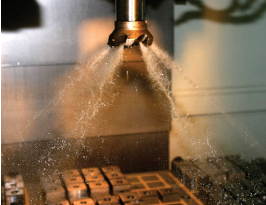
CoolBLAST arbor screw provides coolant path even with non-coolant thru face mills.
