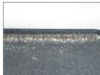
Thermal Cracks (Thermal Wear)
