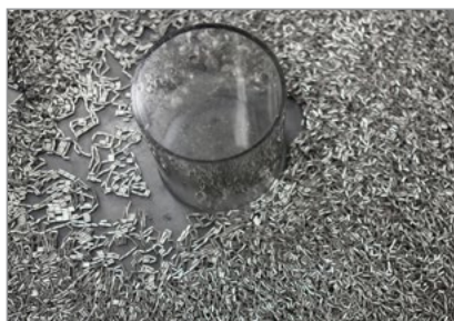
Put media and parts into container and add water and deburring solution.
