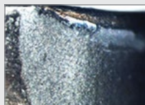
Plastic Deformation (Thermal Wear)
