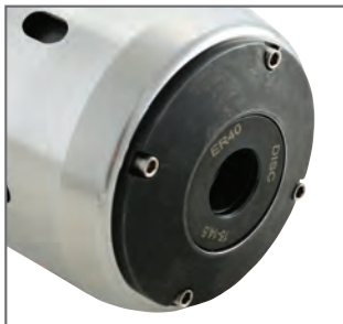
Snap ring into cap. Screw cap to end of milling chuck.
