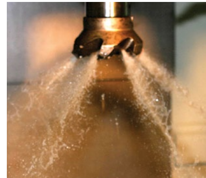
CoolBLAST arbor screw provides coolant path even with non-coolant thru face mills.
