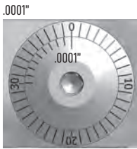
A .0001" Vernier is standard on all finish heads
