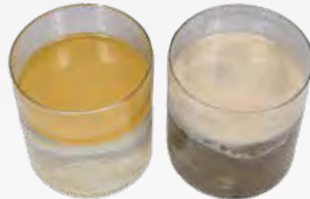
Test samples: Container on left shows untreated oil and water. Container on right was treated with Ultra-Archaea and shows that only lipids were left after the bio-remediation took place. The dark material in the bottom of the container is the clay carrier.
