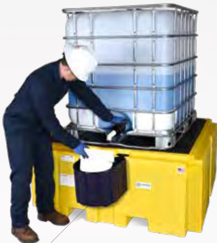
Spills from dispensing that exceed 3 gallons are channeled into the 365-gallon sump through a bulkhead fitting.
