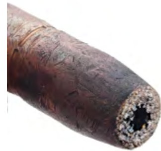
Nozzle fully clogged (not using E-WELD Nozzle)
