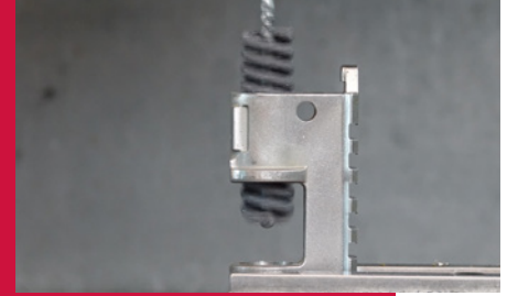
Deburring cross holes in a firearms component.
