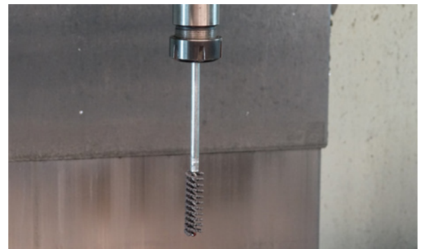
Collet ready CrossFlex brush in a CNC machine.
