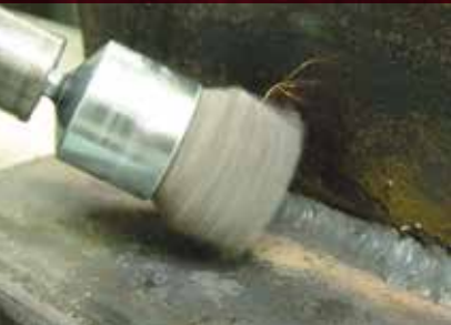
Cleaning hard-to-reach fillet welds with a Controlled Flare End Brush.
