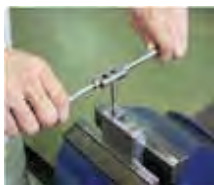
Manual tapping by using tap wrench
